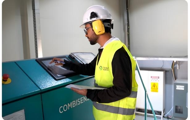
Using a Combisense machine to sort metals at our factory.
